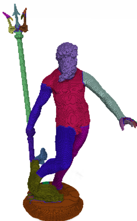
Figure 112: After decomposing a skeleton into simple components, it is possible to propagate the labels of the skeleton throughout the input object in order to obtain a decomposition of the original volume.
