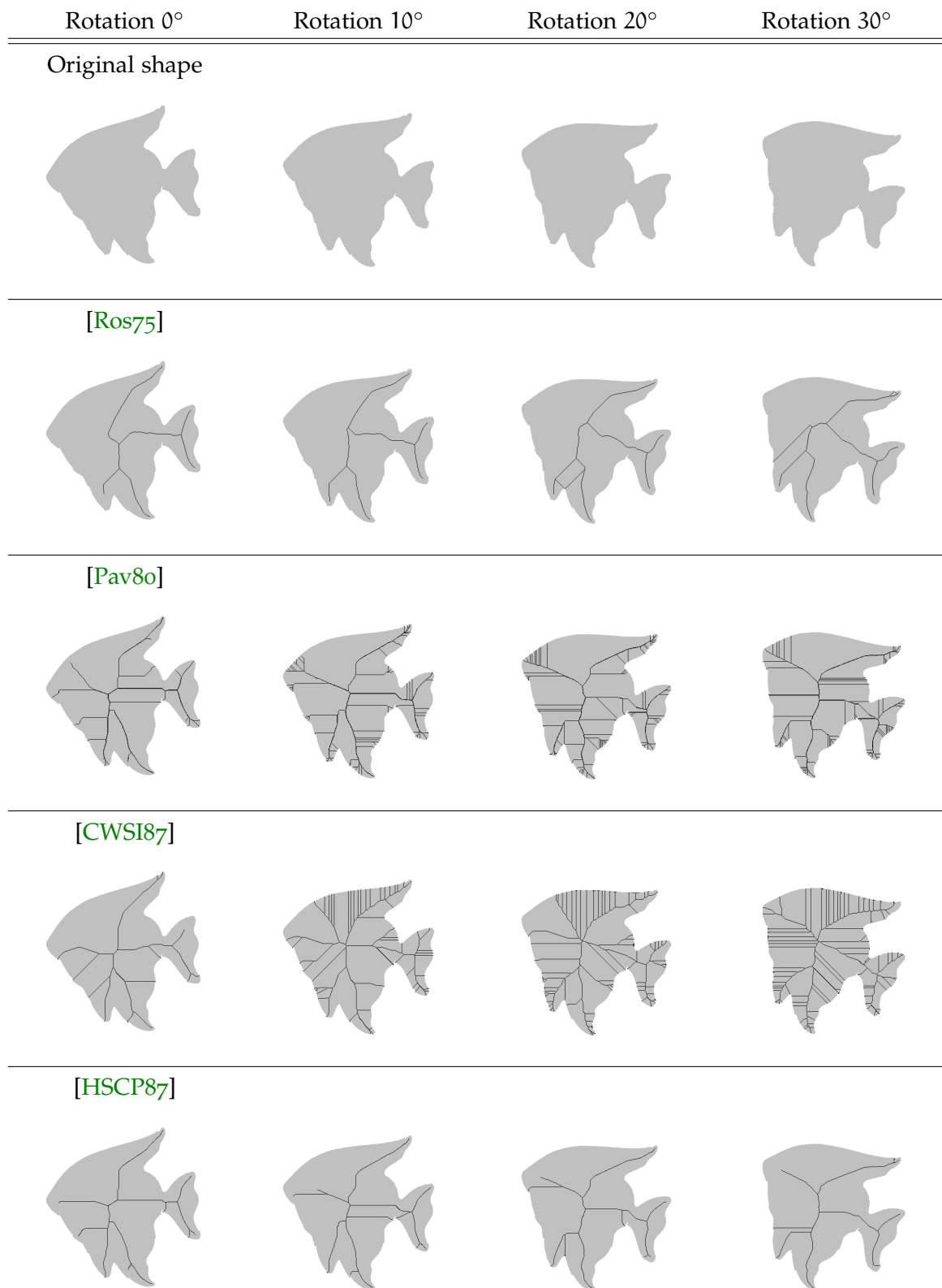
Figure 93: Example of the behaviour of various thinning algorithms to rotation - From left to right, the input is rotated with a greater angle.
